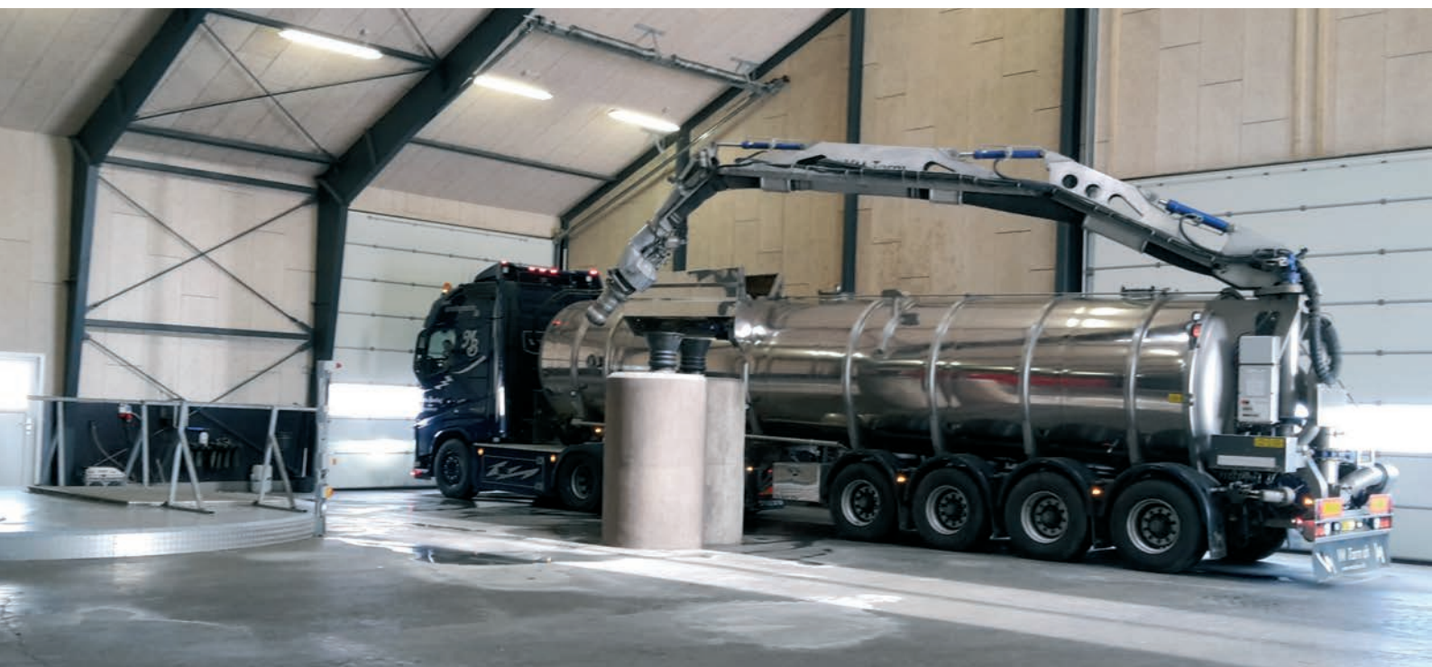
FIGURE 5.9 Truck specially designed for manure transport. PHOTO Food & Bio Cluster Denmark.
