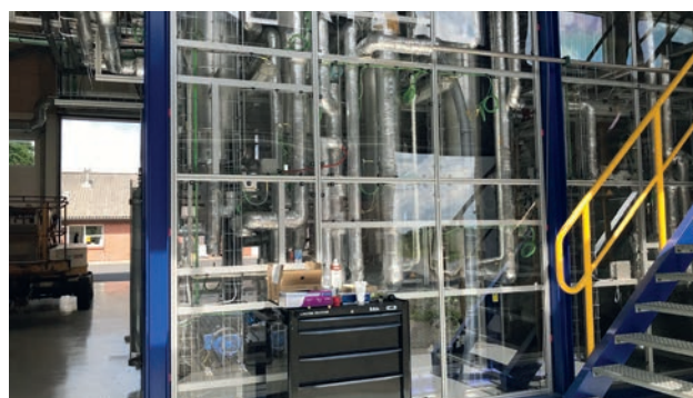
FIGURE 5.10 Conversion of CO 2 and H + to methane at Aarhus University test facilities. PHOTO Food & Bio Cluster Denmark.
